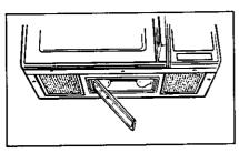
Be sure bulbs to be replaced are cool before removing. Break the adhesive seal by gently unscrewing the bulbs. Replace with 40-watt incandescent bulbs available from your Maytag supplier. High intensity 40-watt bulbs, which are available in supermarkets and hardware stores, may also be used for replacements. Raise light compartment cover and replace screw. Connect electrical power to microwave oven.
