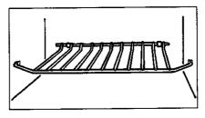
Next, lower the front until the shelf support guides fit **onto** the support guides located at each side of the oven in the front.
