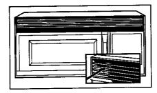
To replace your oven light, first disconnect power at main fuse or circuit breaker panel or pull plug. Remove the top grill by taking out the 2 screws that hold it in place.
