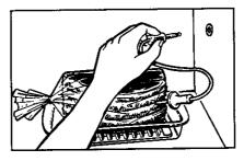
Place meat in oven with probe to the right. Insert cable end of probe firmly into receptacle on oven wall.
