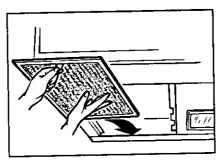
To replace grease filter, slide the filter in the frame slot on the back of the opening.
