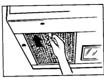
Pull filter upward and to the front to lock into place.
