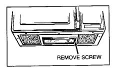
To replace combination cooktop light/night light, first disconnect power at main fuse or circuit breaker panel or pull plug.
