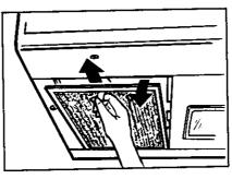
Then pull filter downward and to the front. The filter will drop out.
