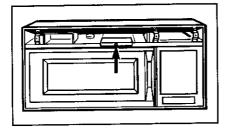
Next, remove the single screw located above door near center of oven that secures light housing. Replace burned-out bulb with a 30-watt incandescent bulb.
